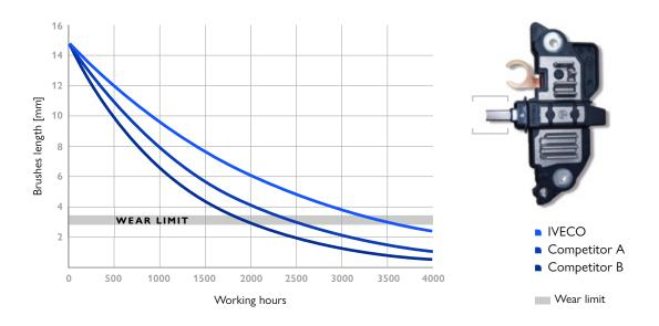
IVECO GENUINE ALTERNATOR TEST RESULTS DEMONSTRATED BETTER PERFORMANCE ALONG THE LIFE CYCLE AND PROVED TO BE MORE RESISTANT TO WEAR.
